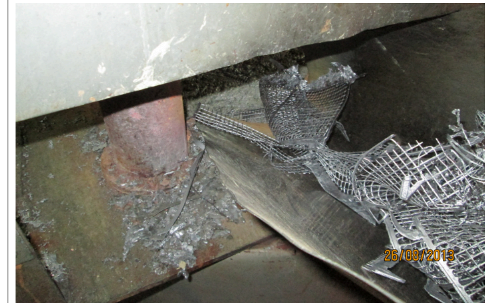
Fig 6a: Blockage of returned castings due to oxide (dross) build up on the surface of the molten alloy.
