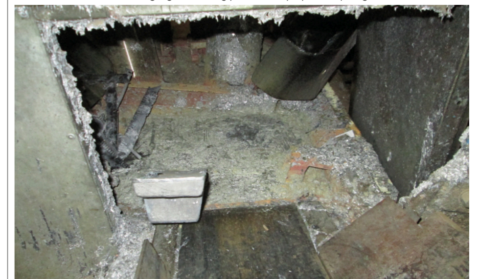
Fig 6b: Clean lead surface exposed after dross removal. The sticky surface layer contains many of the additives that assist the casting, age hardening process and properties of the grid.
