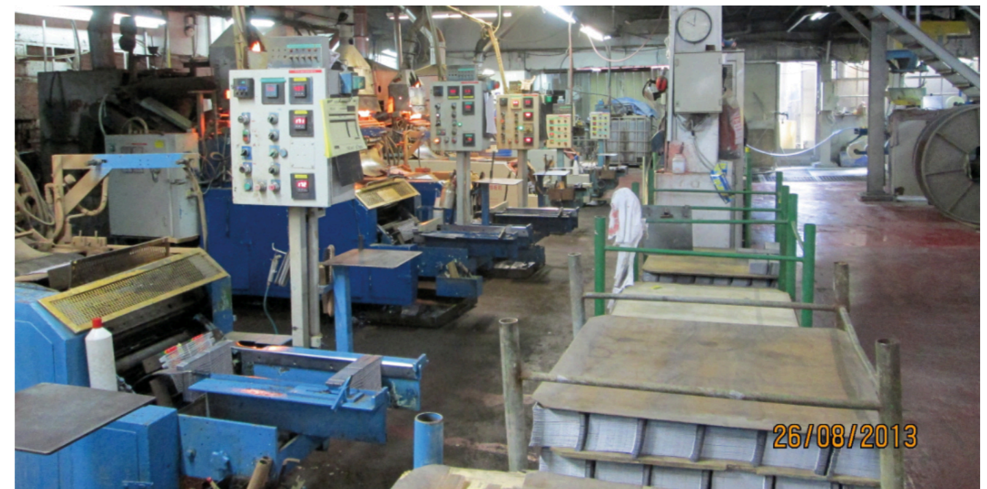
Fig 2: Well run gravity casting shop in a lead-acid battery factory.
