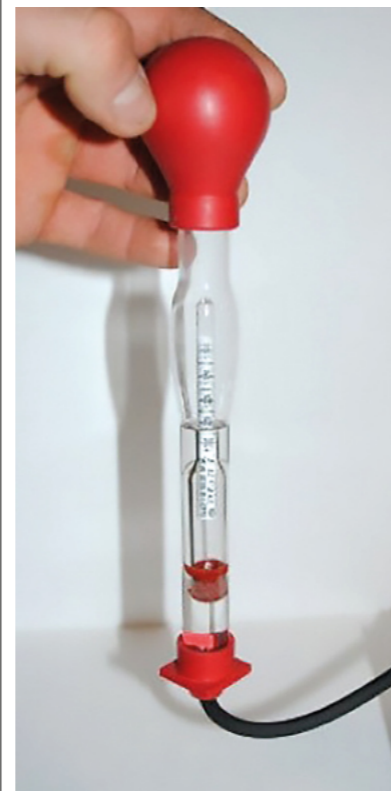
Fig 3: Digital hydrometer commonly used to sample specific gravity and measure electrolyte temperature.
