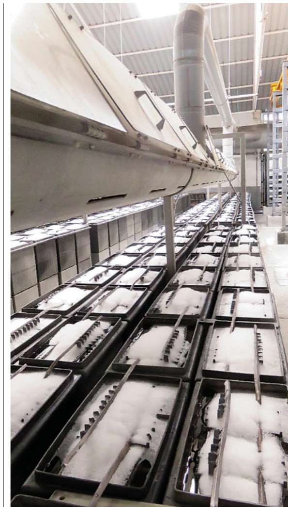
Plate formation line for VRLA recombination batteries
