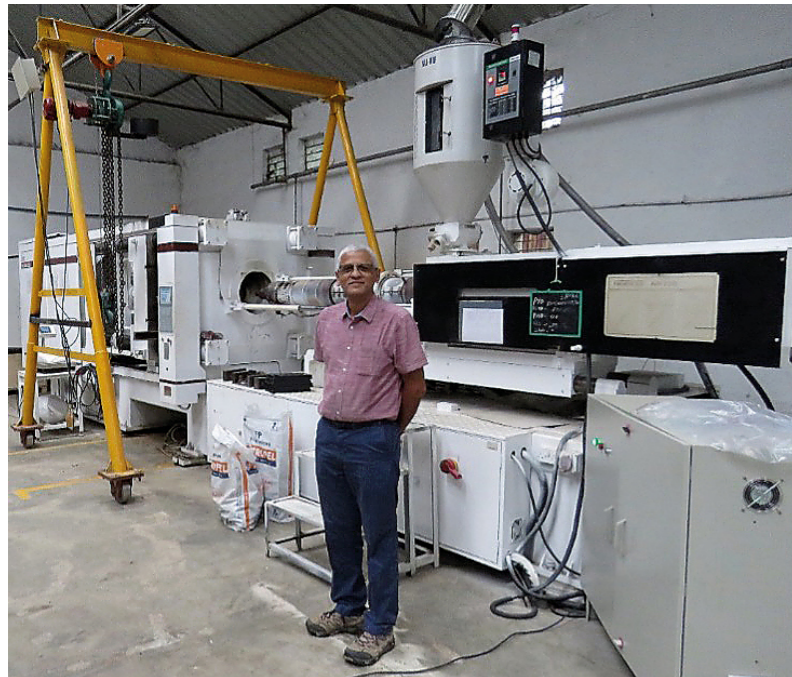
Plastics injection-moulding machine for cell and battery container manufacture
