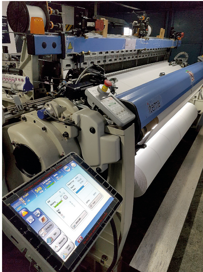
Fully automated, state-of-the-art gauntlet-weaving machine
